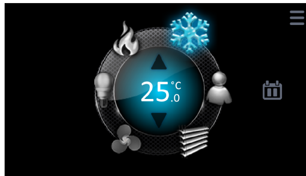
SPACEview showing cooling setpoint
